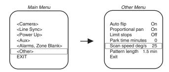
The scan speed is adjustable from 1-40 degrees per second. This occurs in three scan modes: auto, random, and frame scan.
